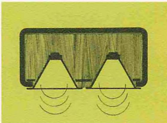
Two permanently sealed tone chamber speaker cabinets house 4 extremely heavy duty 10 inch speakers. Operating on a sealed-in *cushion-of-air*, forward projection of sound reaches the ultimate in musical instrument amplification. In addition, cone excursion is limited for protection against cone breakup.
