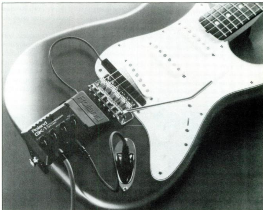
Fig. 1 The GK-1 installed on a guitar. Note the hex pickup between the treble and bridge.
