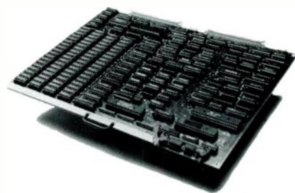
Lexicon's memory expansion board for their 480L digital effects system
