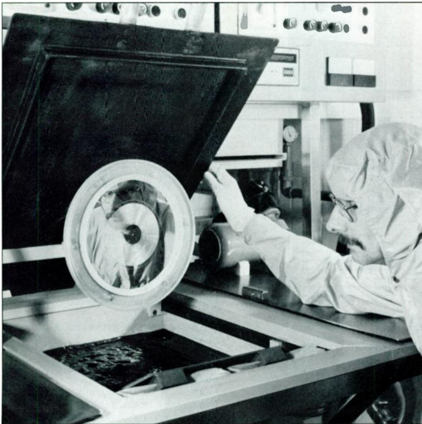
CD plating (transferring the data on the laser-etched glass master to metal stampers) is an electroforming process performed under strict clean room conditions.
