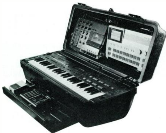
FIG. 1: The briefcase MIDI studio. The slide-out drawer provides access to compact effects devices.
