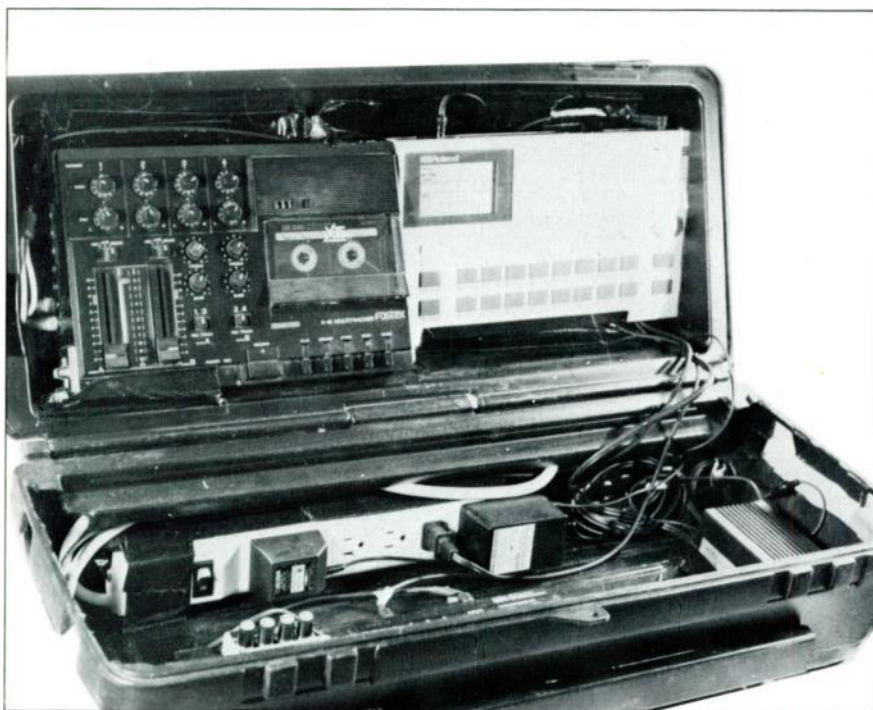
FIG. 2: An AC line filter/power strip mounts behind the effects drawer.
