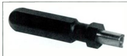
FIG. 1: The Selco collet knob removal tool.
