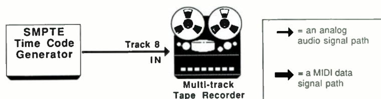
Step 1: Record SMPTE signal on Track 8
