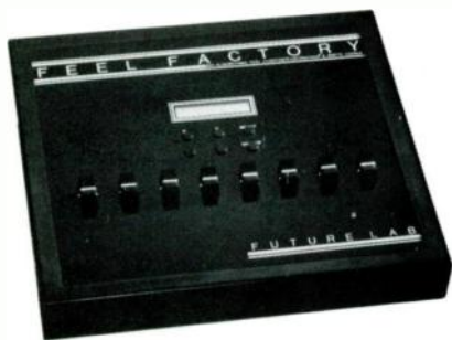
The eight faders on the Feel Factory allow users to change the "feel" of sequenced music.
