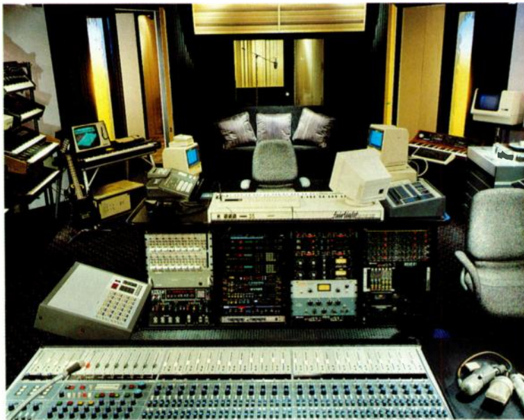
The new demands of electronic music production have changed both the look and design of modern recording studios. Pictured above is Ignited Productions, a 48-track studio in Hollywood, California. Its spacious control room incorporates multiple keyboards and other MIDI instruments (including a dual Fairlight system) into the mixing environment.
