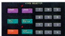
The DSR-2000 stores 60 preset and 40 user voices. All selected by the keypad you see here.
