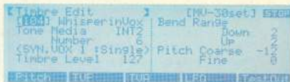
Call up the Timbre Edit display, and you'll have full control over envelopes, LFOs and multi-mode filters.
