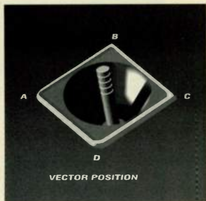
FIG. 1: The Wavestation's joystick controls the balance of as many as four sound elements.
