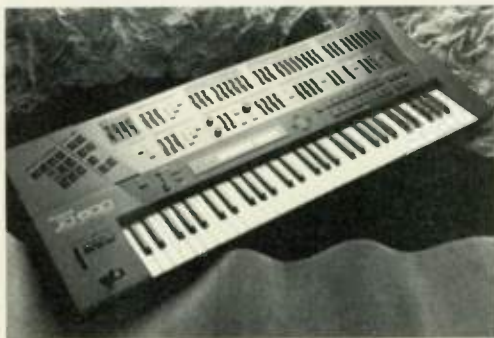
The Roland JD-800 synthesizer's 57 dedicated parameter sliders are active at all times, providing extensive, easily accessed editing capabilities.
