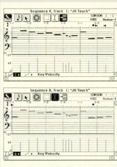
FIG. 4: The top window shows pitches and durations of a musical phrase in piano-roll style. The bottom window shows compressed velocities from the same phrase in bar graph form.
