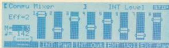
Studio M's Compu-mixer records MIDI volume levels and pan settings for internal and external parts.
