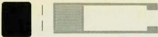
FIG. 1: The Interlink FSR consists of two elements. The square pad on the left is a resistive ink, and the grid on the right is made up of conductive ink. When the pad is placed atop the grid, it forms an element whose resistance varies in proportion to pressure.
