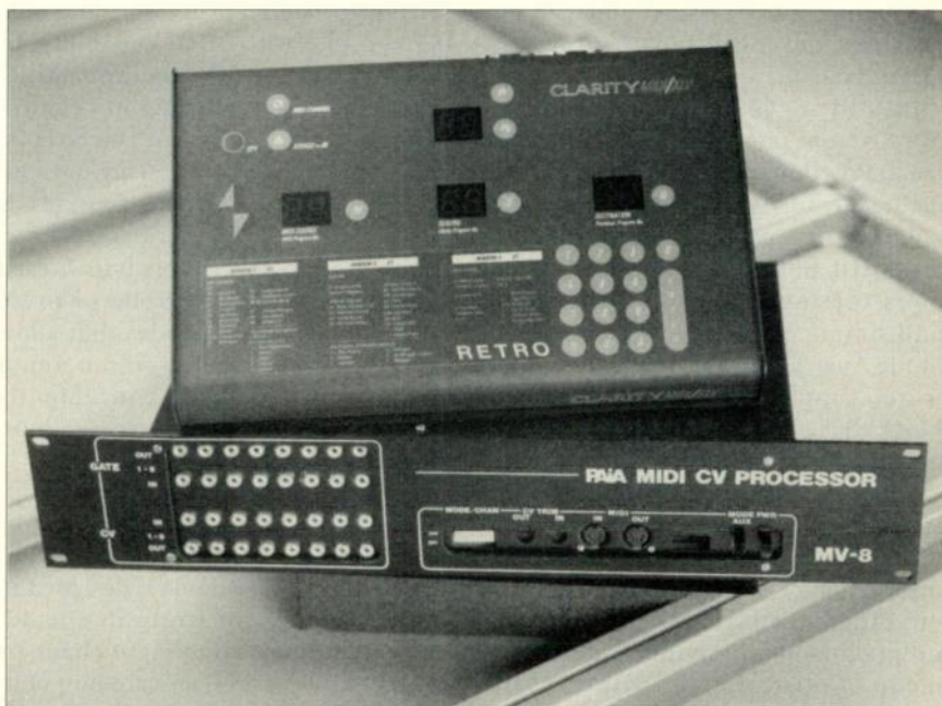
Clarity's Retro MIDI-to-control voltage converter is easy to use and seems aimed at the studio market, while the extremely flexible PAiA MV-8 is better-suited to the experimenter.
