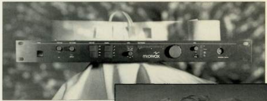
SynchroVoice's MidiVox tracks vocal chord movement, using biosensor pads mounted on a neckband (right). A rack-mount box (above) translates the results into MIDI data.
