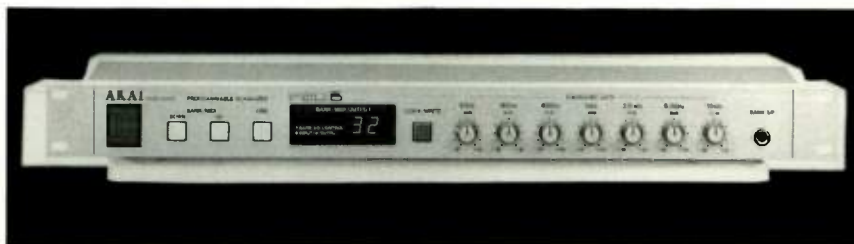
Akai's PEQ6 is a programmable, 7-band, fixed EQ that supports MIDI Program Change commands and accepts parameter changes via SysEx.
