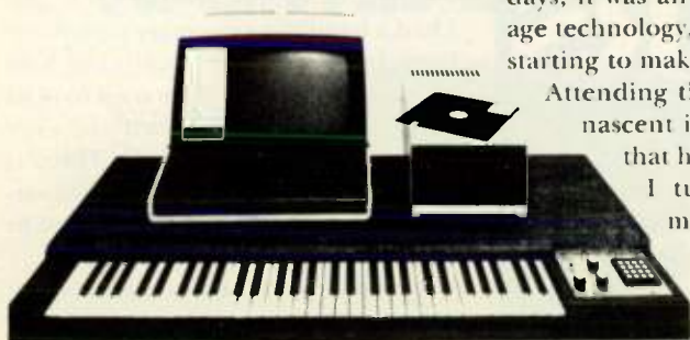
The E-mu Model 4060 keyboard was the first commercial electronic music instrument based on the microprocessor.
