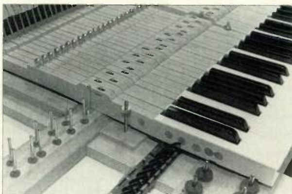
FIG. 2: The KS20 sensors (foreground) use optical scanning technology to track the key travel. Pieces of black plastic—called “Nessies” because they resemble a famous photo of the Loch Ness monster—open and close between the light source and light sensors.
