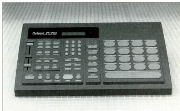
By striking different parts of the Roland R-70's unique Positional Pad (lower right), you can trigger distinct pitches and timbral variations of a sound.
