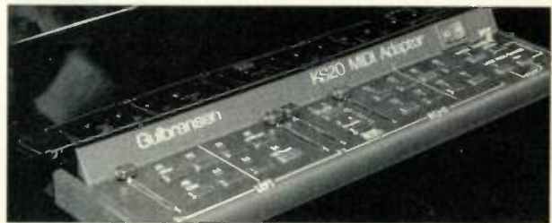
FIG. 1: The Gulbransen KS20's control panel/brain mounts under the left side of the piano keyboard and slides in and out.
