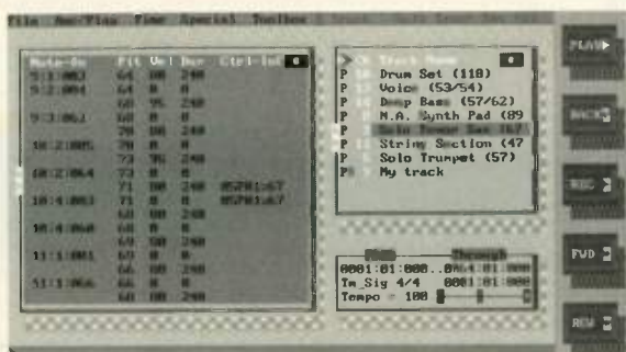
FIG. 2: MusicSculptor provides the ability to copy and delete tracks, mute/play tracks, step-enter note data, and edit data in an event list.
