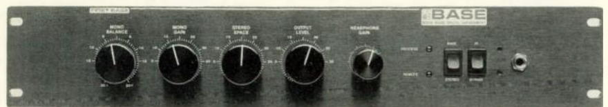
FIG. 4: Gamma Electronics' First B.A.S.E. was the company's first spatial-enhancement product. The system separates the input signal into a mono center image and elements that are exclusively left or right.
