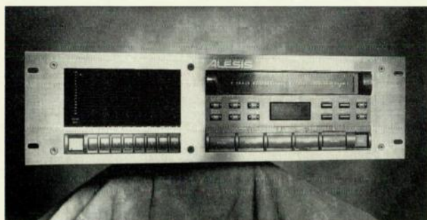
The Alesis ADAT's friendly front panel features familiar tape-transport controls, track-select buttons, and autolocate switches. Metering is handled by the eight 15-segment LED bar graphs at left, and a real-time tape counter is in the center.
