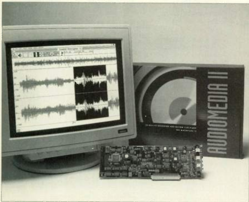
Digidesign's Audiomedia II hard-disk recording system includes Sound Designer II software and the Audiomedia II NuBus card, which has a Motorola DSP56001 processor, A-to-D and D-to-A converters, and digital inputs and outputs.
