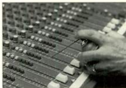
FIG. 5: A blast of compressed air often cleans grungy fader guides.
