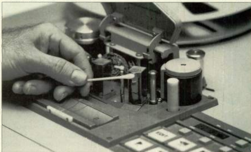
FIG. 1: Cleaning the playback head on a Tascam MS-16 16-track recorder.
