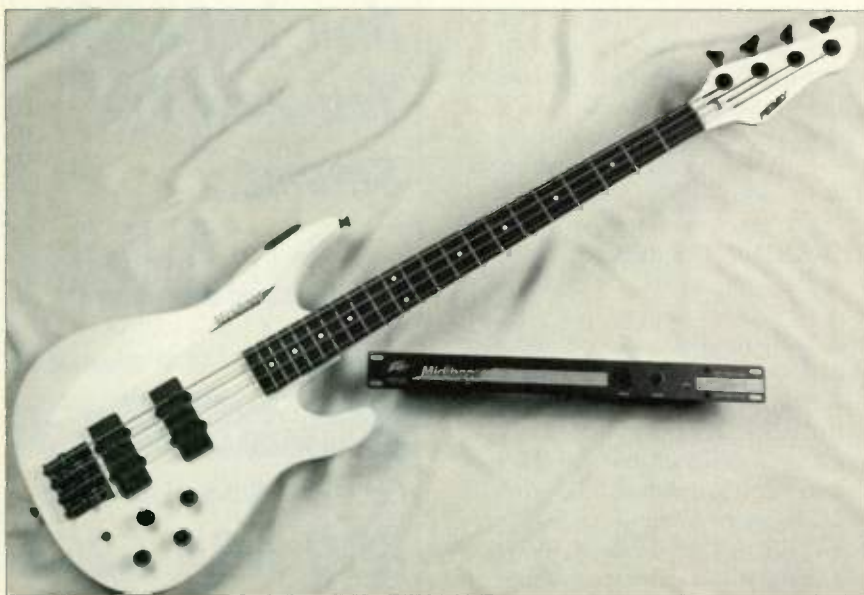
The Peavey Midibase bass-guitar controller uses a combination of wired frets, tension sensors in the bridge saddles, and transducers in front of the bridge to achieve exceptionally fast and accurate tracking and string bends.
