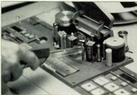
FIG. 3: Demagnetizing heads and metal tape guides helps ensure that oxide gremlins won't mess with your master tape.
