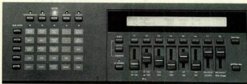
FIG. 1: The sliders under the LCD provide instant access to displayed parameters, as well as certain parameters in Play mode. The Mode Selection Matrix to the left removes much of the confusion inherent in myriad pages of parameters.
