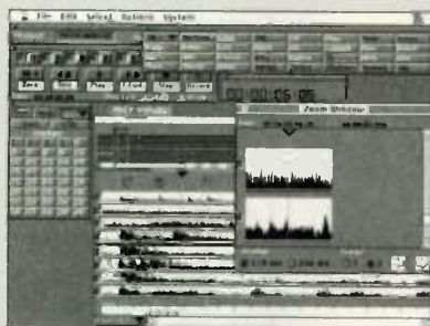
FIG. A: Roland's DM-80-S Multitrack Manager System software for the Macintosh shows all tracks onscreen simultaneously and has a graphic overview of the entire Project above the Track display. The program's release date has not been announced.
