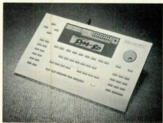
FIG. 2: All functions of the DM-80 are controlled from the DM-80-R remote box. Although it is not included in the system's list price, the remote box is a mandatory purchase.
