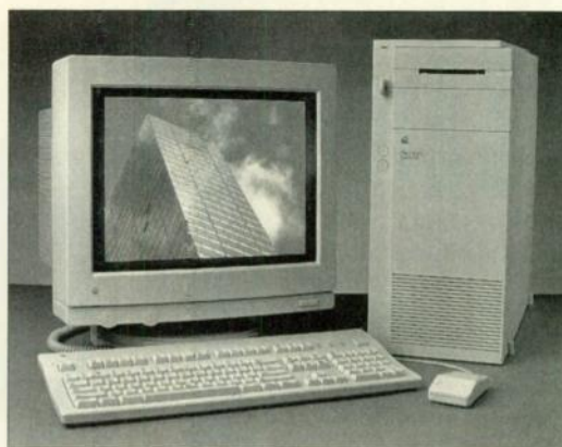
Apple's Quadra 950 offers impressive processing power but requires a Serial Switch system extension to work properly with MIDI.
