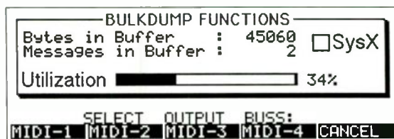
FIG. 2: A 128 KB data buffer can hold SysEx from external MIDI devices for storage to floppy disk or retransmission. The display shows how many messages and bytes of data are in the buffer and how much of the buffer is filled. (Courtesy of Peavey Electronics.)
