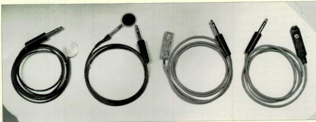
FIG. 4: Four assembled percussion sensors (L to R): piezo, FSR, electret mic without shrink tubing, and electret mic with shrink tubing.
