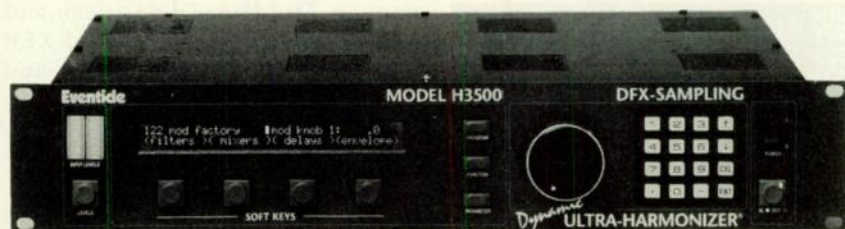
The Eventide H3500 can produce quality chorusing, pitch shifting, ambience, and reverb, but its ability to modulate effects parameters in response to input-signal dynamics sets it apart.
