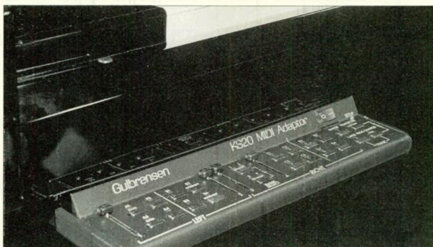
FIG. 1: Gulbransen's KS20 includes a strip of optical sensors installed beneath the keys and a control unit mounted beneath the left side of the keyboard that converts the information to MIDI note and Velocity data.
