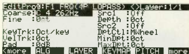
FIG. 2: The frequency of the lowpass filter is edited on the F1 FRQ page.
