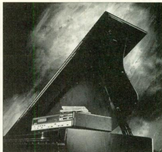
FIG. 4: The PianoDisc PDS-32 system is controlled from a VCR-sized box with a 720 KB floppy-disk drive; the programming buttons; MIDI In, Out, and Thru jacks; and a large LCD display. The system includes a 1-track MIDI sequencer.
