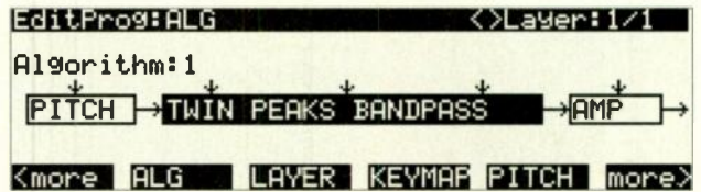
FIG. 1: The K2000's algorithm page, showing one of the instrument's 31 basic sound-design algorithms.
