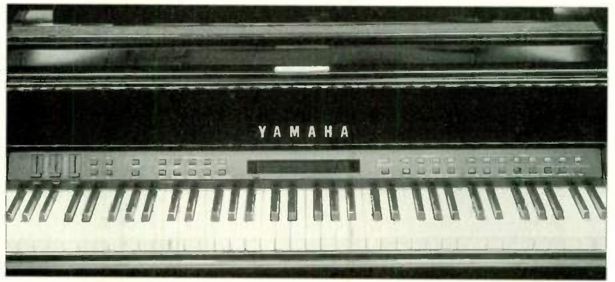
FIG. 2: Yamaha's MIDI Grand is based on Yamaha's 6-foot C3 series and 7-foot, 4-inch C7 series pianos. A 40-character by 2-line display shows the status of its many MIDI features.
