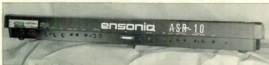
FIG. 1: Unlike its predecessor, the EPS-16 Plus, Ensoniq's ASR-10 has left and right analog audio inputs with an input-level pot. Options (center) include S/PDIF digital I/O and SCSI.
