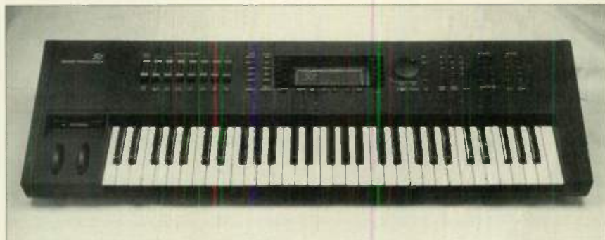
The GeneralMusic S2 offers eight sliders, a built-in disk drive, and a flexible digital filtering system.
