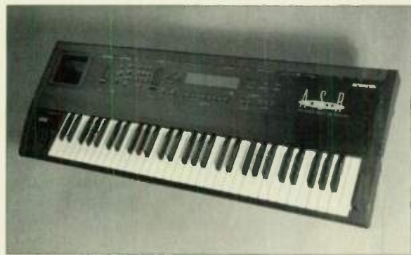
Ensoniq's ASR-10 is a chip off the old EPS-16 sound block, but with significant new features. Noteworthy additions include expandable dynamic RAM, stereo sampling, and an effects processor derived from DP/4 technology.
