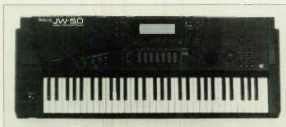
Roland's JW-50 combines a Sound Canvas synth engine with a sophisticated sequencer and numerous real-time controllers.
