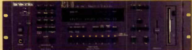
The ASR-10 Rack-Mount has all the power of the keyboard version plus eight outputs and a SCSI interface.
