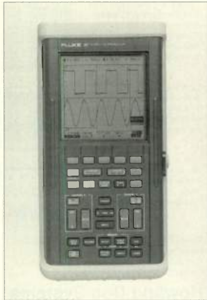
FIG. 1: The Fluke 97 Scopemeter, an LCD mini-oscilloscope with a built-in signal generator, is convenient for testing the phase of audio inputs and outputs.
