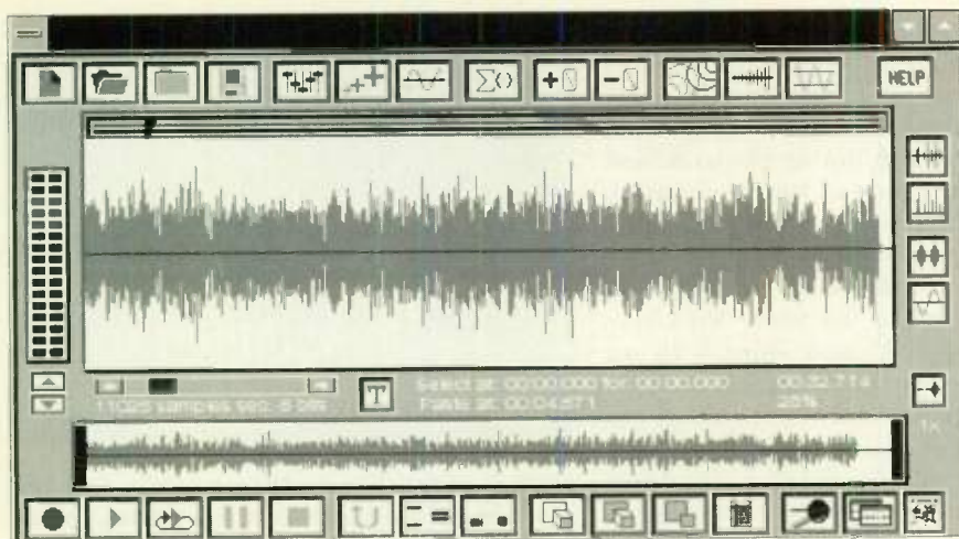
FIG. 4: Sound Impression's Wave Composer is the heart of the program, a "sequencer" for scheduling and combining up to sixteen Wave files. The Wave Composer represents tracks vertically and time horizontally and uses small "segments" to represent Wave files. The display is fairly small and can't be maximized.
