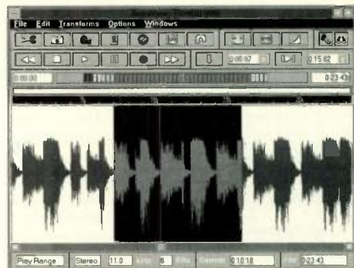
FIG. 3: AudioView's Wave Editor. Windows show the range selection and indicate Play or Edit mode. Information about the file's sampling rate and bit resolution appears along the bottom of the screen. Most—but not all—major editing operations can be accessed from icons. Note that the VU meter is aligned horizontally, rather than the traditional vertical arrangement.
