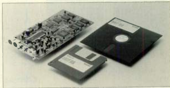
You can add Sound Canvas sounds to a PC-compatible computer with the SCC-1 sound card.
