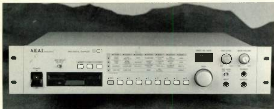
Akai clearly targeted its 8-voice, 16-bit S01 sampler at the entry-level user. The company kept the price down by offering a fixed, 32 kHz sampling rate; minimal editing and continuous-control features; and mono audio output.
