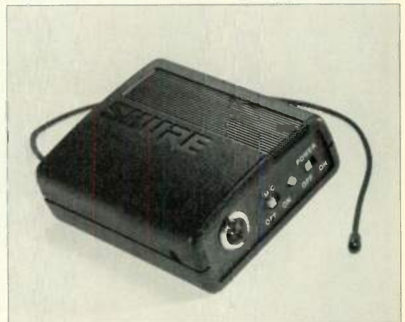
FIG. 4b: The Shure L11 body pack wireless transmitter can be used with headset and lavalier mics. A similar type of transmitter is used for wireless guitar systems.
