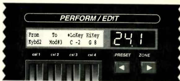
FIG. 1: The asterisk in the Studio 2001's Zone screen indicates that by hitting the Star button, you can access a hidden screen. In this case, the hidden screen lets you set the key range directly from the keyboard. (Courtesy Fatar/Music Industries Corp.)
