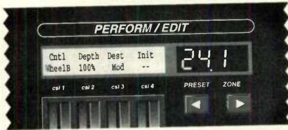
FIG. 2: In the Controls screen and many others, each slider controls the parameter located above it. The LED at right indicates that Preset 24, Zone 1 is being edited; pressing the right-arrow button steps through the other eight Zones in the same screen. (Courtesy Fatar/Music Industries Corp.)
