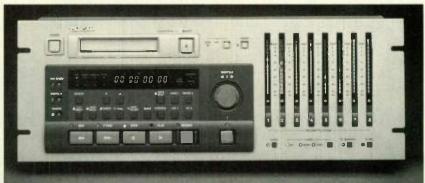
Tape-based, digital multitrack recorders, such as the Alesis ADAT and Tascam DA-88 (shown), offer inexpensive data storage compared to hard-disk systems. Users can just let the tape run and record multiple takes of a work without fretting over available storage space.
