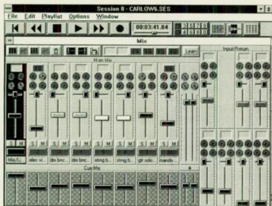
FIG. 2: The Mix screen, with channel 1 record-enabled. Note EQ assigned to channels 2 and 8. The groups are color-coded.
