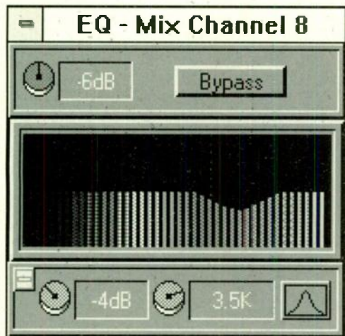
FIG. 3: The EQ window opens when an EQ module is double-clicked. The parameter values can be selected from a preset list but are not continuously variable.
