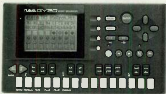
The QY20 includes an 8-track sequencer, multitimbral sound module, and a well-designed user interface with 128 x 64 LCD display, 2-octave keyboard, and cursor-control cluster.
