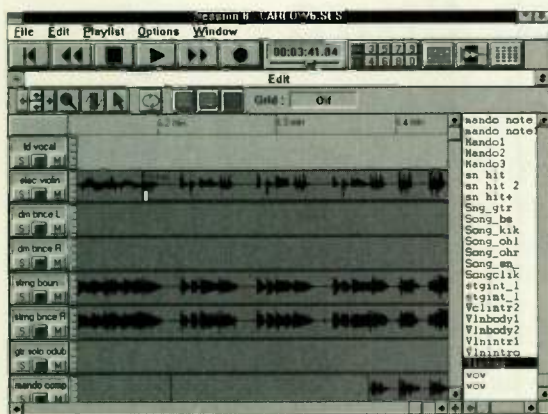
Digidesign Session 8's Edit screen. Waveform overviews have not yet been computed for the drum bounce on tracks 3 and 4. The gray blocks on tracks 7 and 8 are Silence regions.
