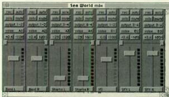
FIG. 1: Digidesign's Pro Tools 2.0 features an integrated recording and editing environment. The Mix window lets you set levels, panning, EQ, and more for each track in a Session.
