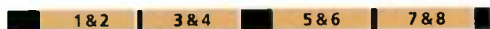
An 8 track, 8mm recorder's helical scan: there are only four audio data blocks, forcing each track to share a block with another.
