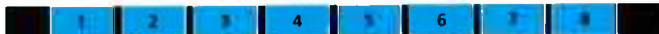
An ADAT's helical scan: ADAT tracks are safely separated into 8 discrete data blocks. (Both vertical dimensions enlarged for clarity)
