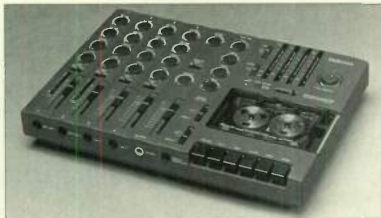
The Tascam Porta 07 includes a 4-track cassette deck, 4 x 2 mixer, dbx II noise reduction, and excellent sound.
