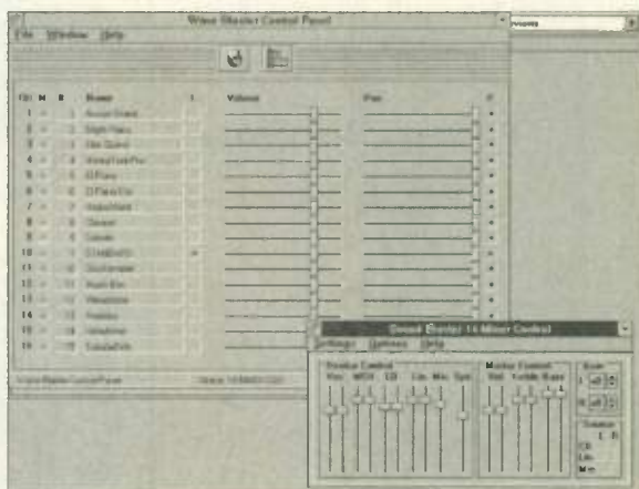
FIG. 2: A specialized mixer and configuration panel for the Wave Blaster works in conjunction with the sound-source mixer for the Sound Blaster 16 ASP.
