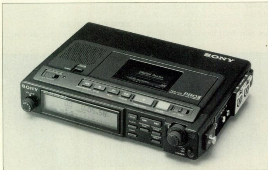
FIG. 2: A portable DAT, such as Sony's TCD-D10 Pro II, can be used for more than just recording stereo masters. You can field record samples and live gigs, do computer data backup, and use it as a stand-alone A/D or D/A converter.
