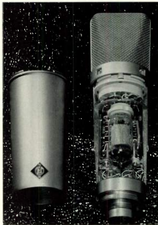
Tube microphones are prized for their warm reproduction. Using a mic such as the Neumann U67 (shown) can help digital tracks sound more full-bodied. The classic Neumann tube mic, the U47, hasn't been manufactured since the 1950s, and used models command a price of $3,000 or more.
