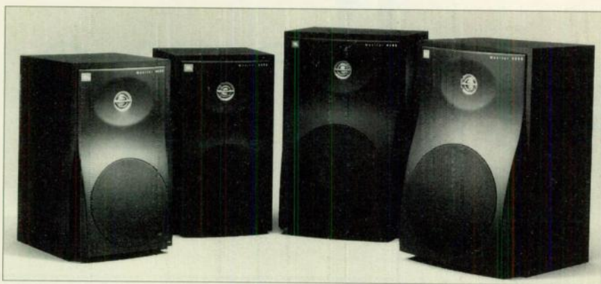
JBL's 4200 series features a molded, "Buddha-belly" front-baffle shape that reduces diffraction effects and aligns the voice coils of the tweeter and woofer so frequencies from the two reach the listener simultaneously.
