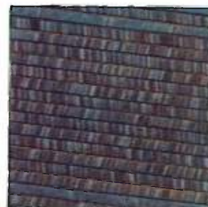
The 8mm's 20-micron tracks squeeze more data into the same area, with little room for error.
