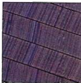
ADAT's wide 100-micron tracks offer an extra margin of safety for digital audio.
