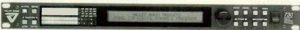
Valley Audio's new Model 730 Digital Dynamics Processor allows MIDI control of its fully digital compression, expansion, limiting, and noise-gate functions.
