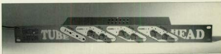
In the EM TubeHead, the tubes are mounted horizontally to fit in a single-rackspace case.
