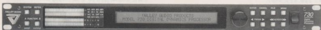
Valley Audio's new Model 730 Digital Dynamics Processor allows MIDI control of its fully digital compression, expansion, limiting, and noise-gate functions.
