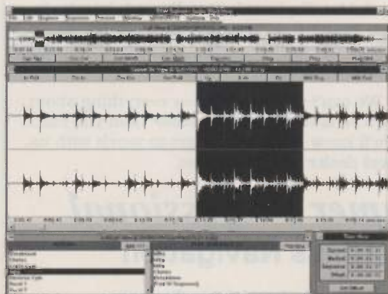
FIG. 1: SAW's opening screen. The Full View window provides an overview of the entire active soundfile, while the SoundFile View provides a standard waveform display. You assemble the Regions in the EditList View, while Time View indicates your cursor position's location in time.
