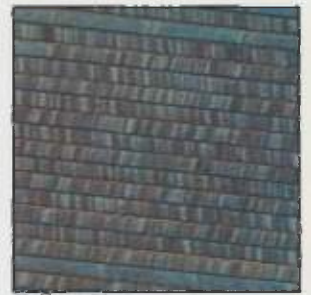
The 8mm's 20-micron tracks squeeze more data into the same area, with little room for error.
