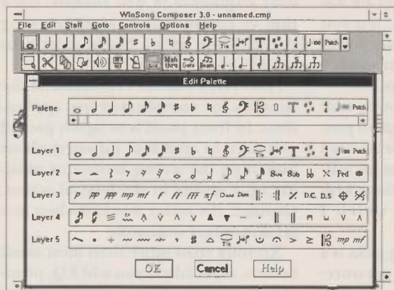
FIG. 1: If you don't like the arrangement of icons in Composer 's toolbar (shown at the top of the screen), you can change their arrangement by dragging them around in the Palette Editor. The arrow buttons at the top right scroll the toolbar through its five different layers.
