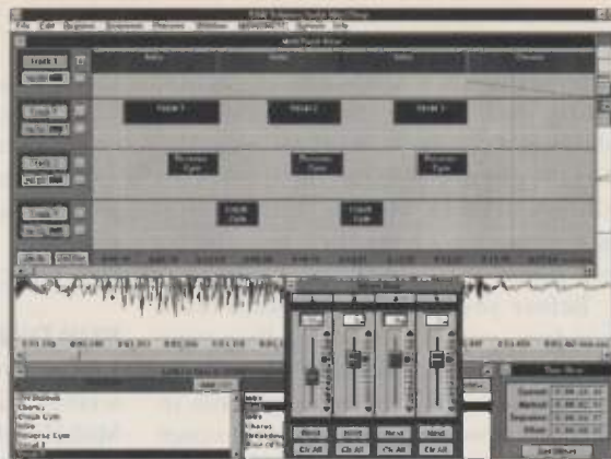
FIG. 2: In the MultiTrack View window, Regions appear as small, horizontal bars that can be moved to any starting point. You can't overlap Regions in the same track, or move them across tracks.
