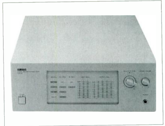
Yamaha's forthcoming CBX-D5 will work in conjunction with digital-audio sequencers, such as MOTU's Digital Performer , to give four independent audio tracks to MIDI sequences.
