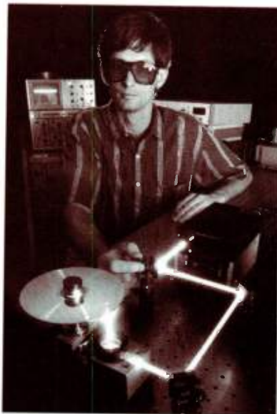
FIG. 1: Dr. William J. Kozlovsky, research staff member at IBM's Almaden Research Center, demonstrates a compact, blue-laser, MO storage system. (Photo courtesy IBM Corp., Research Division, Almaden Research Center.)
