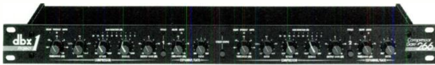
Combination compressor/noise gate units, such as the dbx 266, allow recordists the ability to maximize signal levels and shut out the majority of annoying environmental noises.
