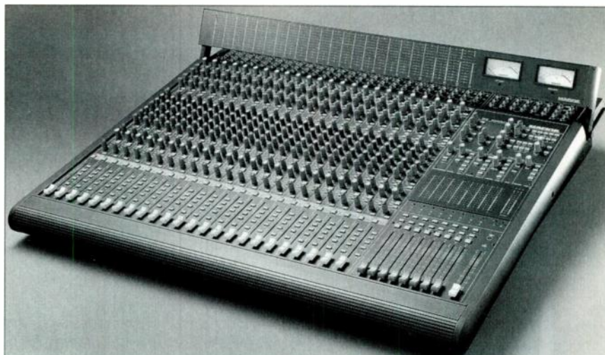
The Mackie 8•Bus series of in-line consoles offers 4-band EQ and a Mix-B section that allows each channel strip to return two signals simultaneously. With group and effects returns, this means you can get approximately 60 signals into the 24 x 8 x 2 model.
