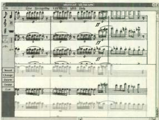
FIG. 1: MNOD editing tools are located in an icon tree (left) and help fine-tune files before conversion to MIDI. The music in this example is the TIFF file included with the program.
