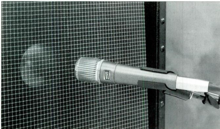
Supercardioid dynamic mics, such the Shure Beta 57, are perfect as all-purpose workhorses for close-miking situations. These types of microphones are less sensitive to sounds emanating from the back and sides.
