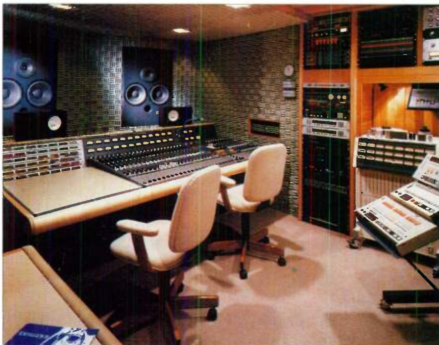
FIG. 3: Absorption can help your studio produce truer sound by diminishing sound reflections and combating frequency anomalies. Sonex (shown on the walls and ceiling near the above mixing station) is a commercially available absorptive material that can be used to completely cover reflective surfaces.
