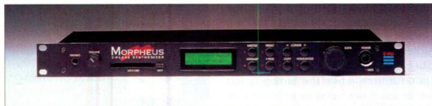
The Morpheus Z-Plane Synthesizer features the ability to "morph" between up to eight different complex, multiband filters.
