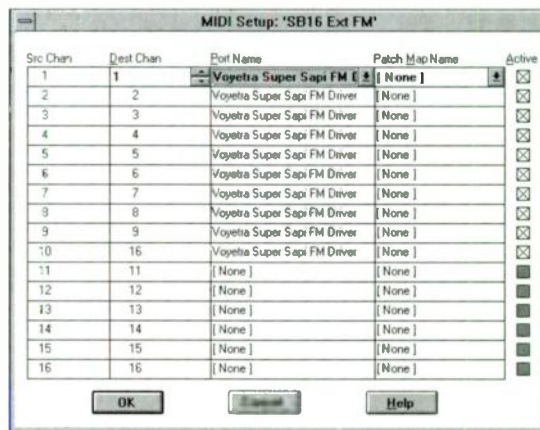
FIG. 2: The Setup window of MIDI Mapper lets you assign MIDI channels and Patch Maps for your sound card and other MIDI devices.
