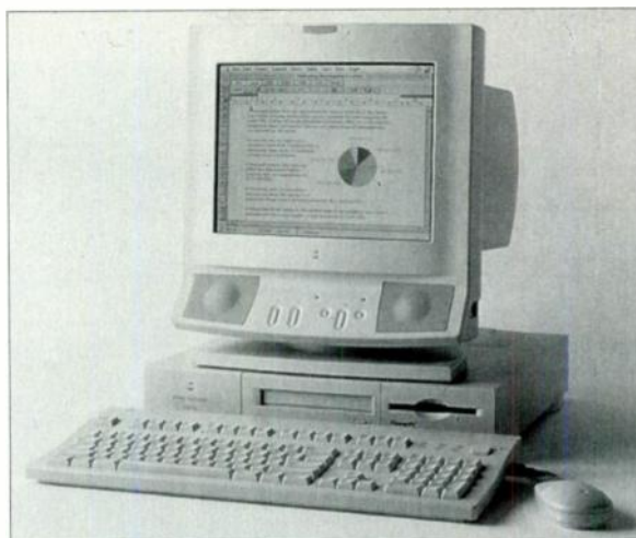
The Power Macintosh 6100/60 gets you into the latest technology for just $2,000, including monitor, keyboard, and 8 MB of RAM. The 6100/60's most noticeable limitation is its one 7-inch NuBus slot.
