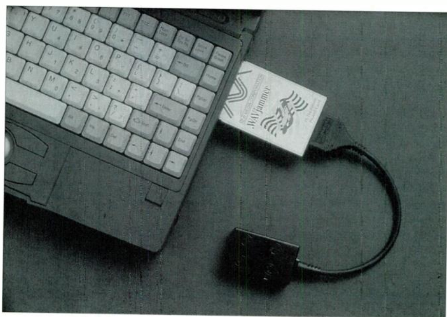
FIG. 3: New Media's .WAVjammer PCMCIA card adds Sound Blaster compatibility to laptop computers, complete with FM synthesis and 16-bit digital-audio recording.
