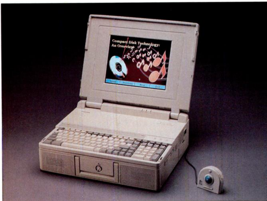
Heavy but powerful, the 17.1 pound Toshiba T6600C lunch bucket features built-in stereo speakers, 520 MB hard disk, and room for an internal CD-ROM drive.
