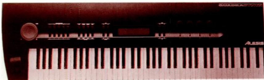
The QuadraSynth features 64-voice polyphony, 16-part multitimbral capability, 76 keys, 16 MB of sample ROM, and an optical ADAT interface. The volume knob resembles a hockey puck, and all controls are located in a central trough. The design is clean and uncluttered.
