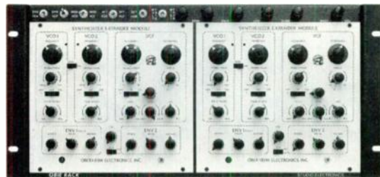
Oberheim's Synthesizer Expander Module (SEM) is difficult to emulate because of its state-variable VCF, which can act as a highpass, lowpass, or bandpass filter.
