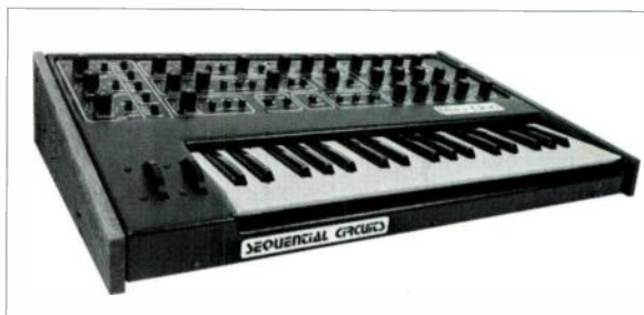
Sequential Circuits' Pro-One has a classic hard-wired mono synth architecture. Two VCOs are summed in a mono mixer and routed through a resonant filter and VCA, each with dedicated, 4-stage envelope generators.
