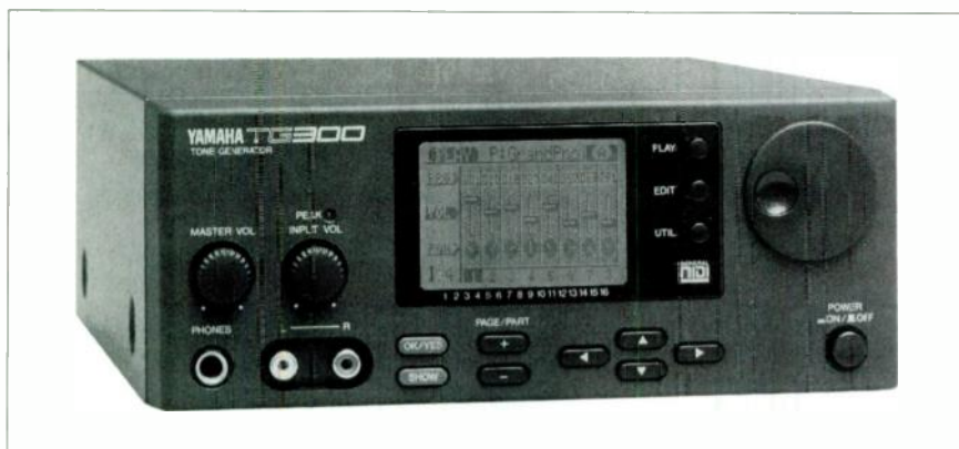
Yamaha's TG300 offers better sounds, more programming power, and more MIDI control than the company's previous GM modules, yet is easy to use. Its built-in PC/Mac interface is a nice bonus.
