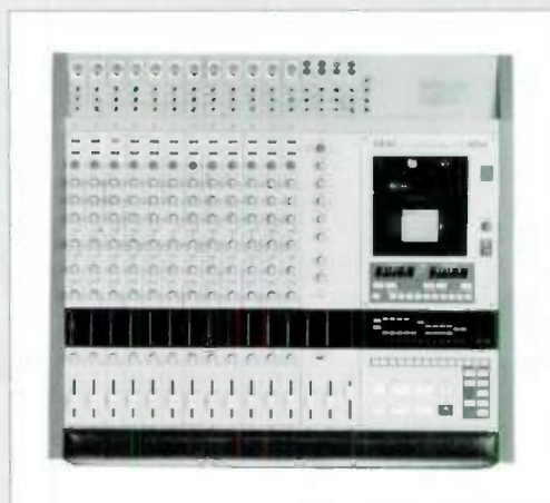
The Akai MG1214 that Maguire, Hall, and Hogan use to demo music for Thunder in Paradise is an integrated 12-channel mixer/14-track recorder that uses custom 1/2-inch cassette tapes. The MG1214 was manufactured from 1986 to 1989, and yes, Akai still stocks the tape.
