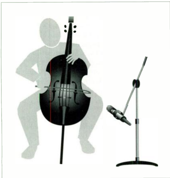
FIG. 1: Placing a condenser mic off-axis from the cello sound-hole can reproduce full low frequencies.
