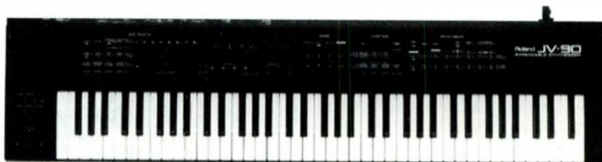
The Roland JV-90 Expandable Synthesizer produces clean, full sounds for a fair price. With the addition of voice-expansion and wave-expansion circuit boards, its polyphony and waveform ROM can be doubled and its multitimbral capability tripled.
