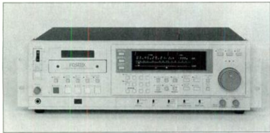
Cleaning tapes provide a blissfully easy method for scrubbing up the rotary heads of DAT recorders such as the Fostex D-10.
