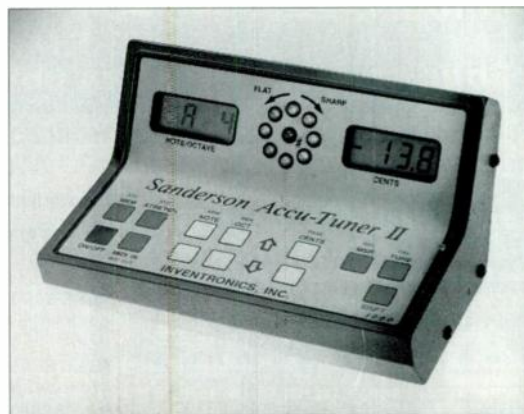
FIG. 1: Sanderson's digitally controlled Accu-Tuner allows extremely accurate custom tuning.
