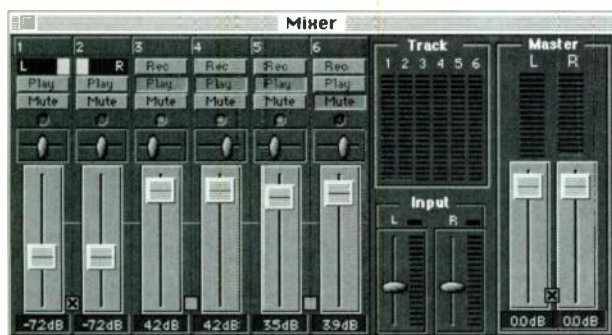
FIG. 1: Alaska Software's DigiTrax includes a Mixer window that emulates a traditional analog mixing board, with input channels, a meter bridge, and master input and output faders. The program provides simple hard-disk recording for the Mac AV and other ARTA-compatible Macs, with few frills.
