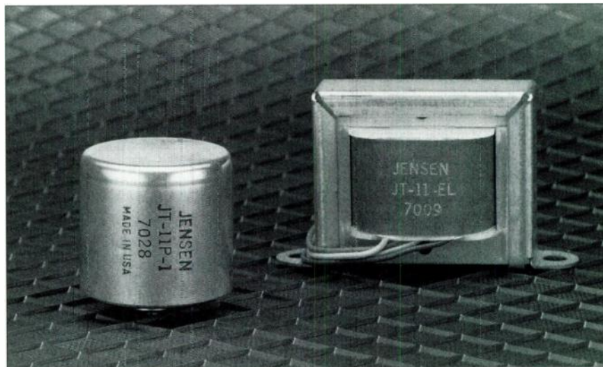
Jensen's JT-11P-1 (left) is a top-notch, professional-quality transformer that can handle up to +19 dB before it hits 1% distortion at 20 Hz. However, you have to drill out a case for the connectors and wire them yourself.
