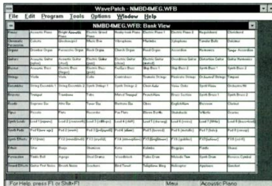
FIG. 4: WavePatch allows the user to work with the synthesizer on many different levels. The Bank View displays all the Programs that are currently loaded. To edit a specific Program, double-click on its name, and move to the Program View window.
