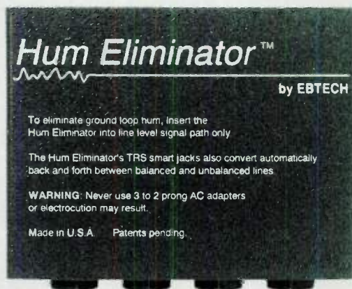
Ebtech's Hum Eliminator provides two low-cost isolation transformers with balanced, 1/4-inch I/O.
