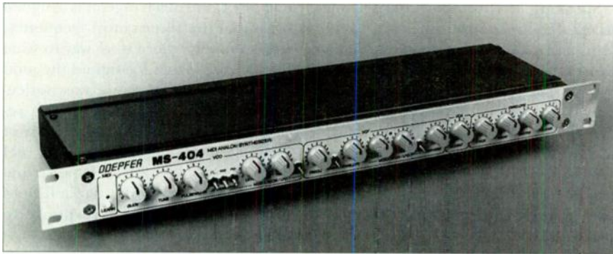
The Doepfer MS-404 monophonic, analog synthesizer module offers excellent analog sound, but it has few special features and no patch memory.
