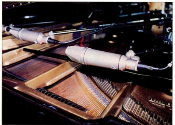
FIG. 2: This is the final placement of three Neumann U 87 mics over the grand piano. Note the consistent off-axis tilt.
