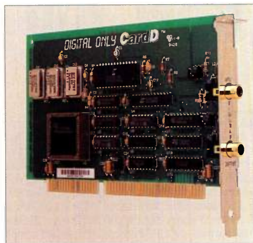
FIG. 1: The Digital Only CardD provides digital ins and outs for direct connections to a CD player or DAT machine.
