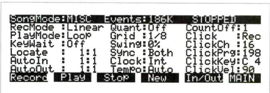
FIG. 6: The sequencer Misc page lets you specify many record and playback parameters. (Courtesy Kurzweil)
