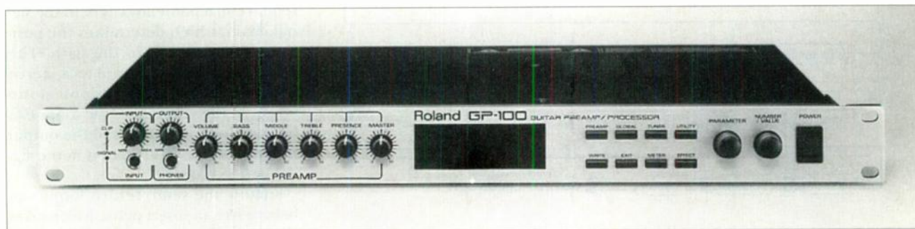
The Roland GP-100 produces high-quality guitar effects, including a wide variety of modeled amp and speaker simulations.
