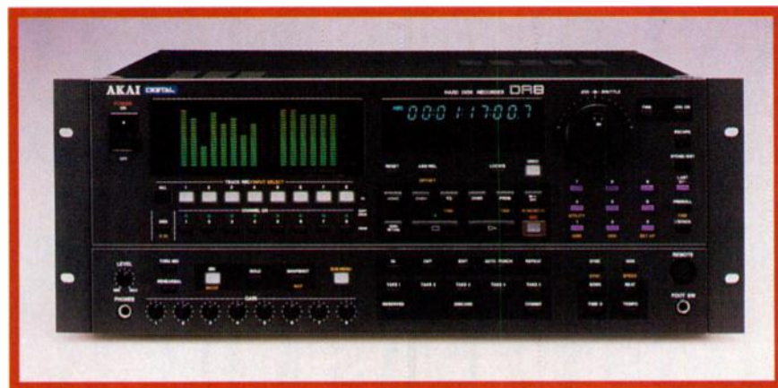
Dream Date #1: Modular hard-disk recorders, such as Akai's DR-8, deliver the benefits of random-access recording without the computer but are usually hampered by dinky user interfaces.
