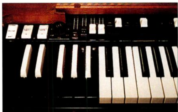
FIG. 1: The drawbars on the B-3 let you mix the volumes of fundamentals and harmonics, giving you a practically unlimited variety of sounds. Also shown here are the controls for the Vibrato and Chorus effect.
