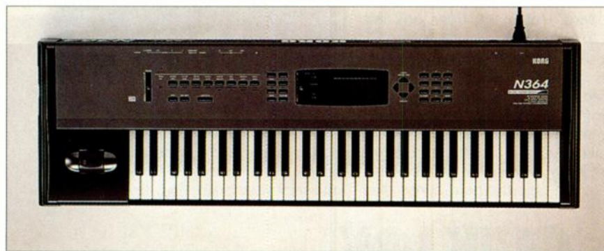
Korg's 61-key N364 keyboard workstation and its sibling, the 76-key N264, use the same PCM-based synthesis engine found in the X-series synths but add a bank of 200 cool new Programs and Combinations, a nifty arpeggiator, and some flashy, rhythmically looped Multisounds.
