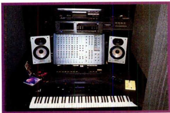
The A/V program's mixing station sports a Studiomaster Star System console (with an Ensoniq KT-76 in the foreground). The console's upright configuration suits the tight quarters perfectly.
