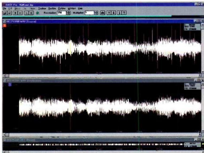
FIG 1: Clicks and pops are clearly visible as narrow amplitude peaks in the top waveform. After I ran the DeClick filter, they were completely eliminated, as shown in the bottom waveform.
