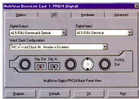
FIG. 1: Many cards use software to control the type of digital I/O. This is the digital I/O control window of Adb's Driver Link software for the Multi!Wav Digital PRO24.
