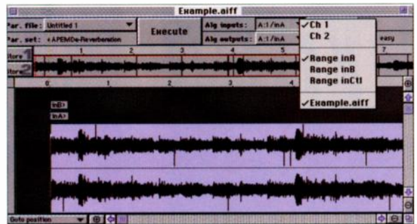
FIG. 3: In SonicWorx Artist , you route sounds between plug-ins by selecting a portion of the sound in the Waveform Editor and assigning its destination using the routing flip menu at the top of the Waveform Editor window.
