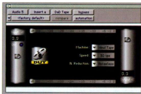
FIG. 3: The DaD Tape interface allows you to select from several tape machine types, tape speeds, and noise-reduction modes.
