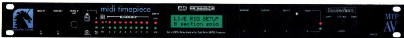
The MIDI Timepiece AV combines sophisticated MIDI interface/patch-bay features with an array of useful audio/video synchronization capabilities.
