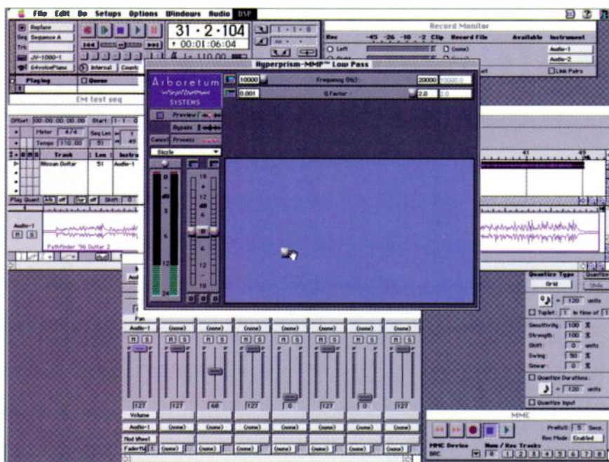
FIG. 1: All Adobe Premiere plug-ins are called up from the Premiere Plug-Ins folder submenu of the DSP Menu. Here, a lowpass filter in Arboretum's Hyperprism-MMP is about to be applied to a guitar track.
