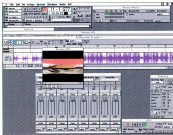
FIG. 2: This QuickTime movie and its audio track, which has been extracted for editing, are locked together. As you scrub audio or enter SMPTE values in the control window, the movie chases to the exact audio location.
