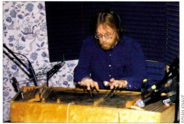
FIG. 2: Michael Masley's cymbalom is stereo recorded with a matched pair of Neumann KM 184 small-diaphragm condenser mics. The Shure SM 58 is patched into a DigiTech Talker vocal synthesizer. From there, the signal goes onto a separate track, giving the mix engineer and effects track for added options.
