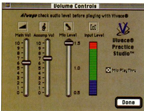
FIG. 1: The Volume Controls dialog box lets you set the main volume, accompaniment volume, and mic input level, which is indicated by the adjacent meter. The Mic Play Thru checkbox mixes the mic signal with the accompaniment, but it also introduces a loud buzz into the signal.
