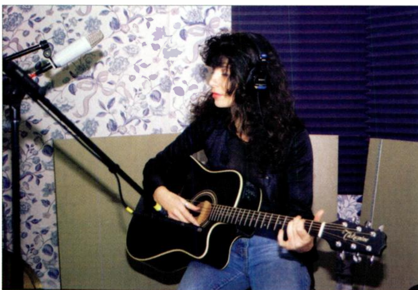
FIG. 1: An AKG C 460 and Røde NT1 capture a stereo image of Lygia Ferra's Takamine EF36 guitar. Several mics were auditioned, but these were chosen because they played down this particular guitar's bassy response, making for a brighter sound that worked better in the mix.
