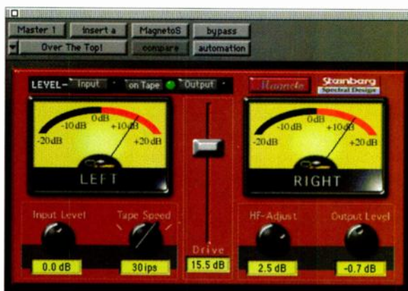
FIG. 4: Steinberg's Magneto plug-in adds the warmth of analog recording to digital audio (TDM version in stereo shown).
