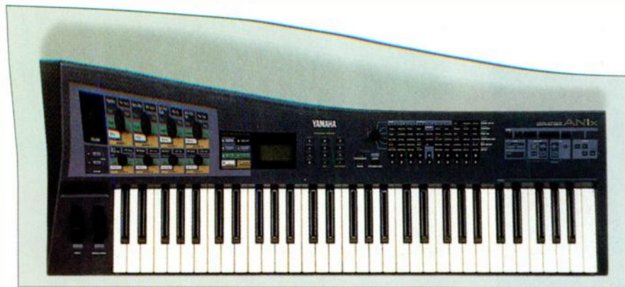
FIG. 1: Yamaha's AN1x synthesizer offers an array of knobs and sliders to control patch parameters in real time.
