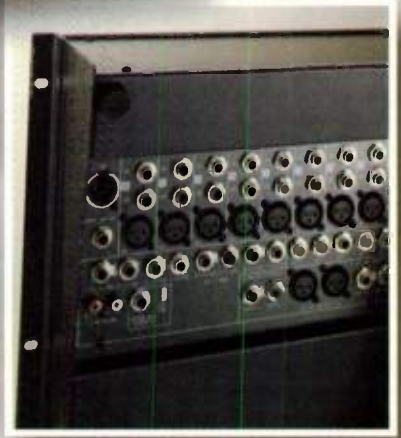
16. All metal rear connector panel repositions for rackmount use
