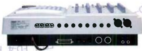
The back panel of the FD-4 shows off its tremendous flexibility. Balanced XLR Mic inputs, optical S/PDIF and MIDI in and out, SCSI-II plus standard analog ins and outs make the FD-4 adaptable to any application.
