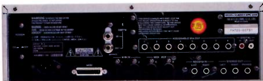
FIG. 1: The rear panel includes stereo audio inputs and main outputs, a headphone jack, a SCSI port, and two sets of MIDI In and Out jacks. Optional expansion boards can add S/PDIF digital I/O and eight more analog outputs as well as SMPTE sync I/O.
