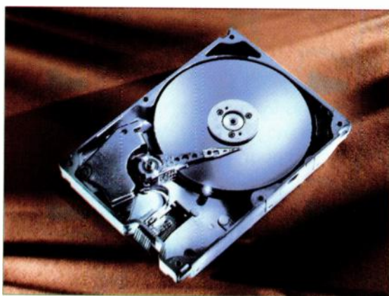
Because of their speed and reliability, fixed hard drives, such as this Quantum Fireball (shown with the top removed), are still the preferred storage devices for most musicians.
