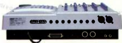
The back panel of the FD-4 shows off its tremendous flexibility. Balanced XLR Mic inputs, optical S/PDIF and MIDI in and out, SCSI-II plus standard analog ins and outs make the FD-4 adaptable to any application.
