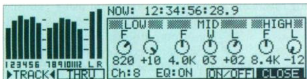
FIG. 2: All EQ settings for a single channel can be viewed using the optional Strip mode. The 3-band EQ shown here can be used on a maximum of six simultaneous tracks/channels.
