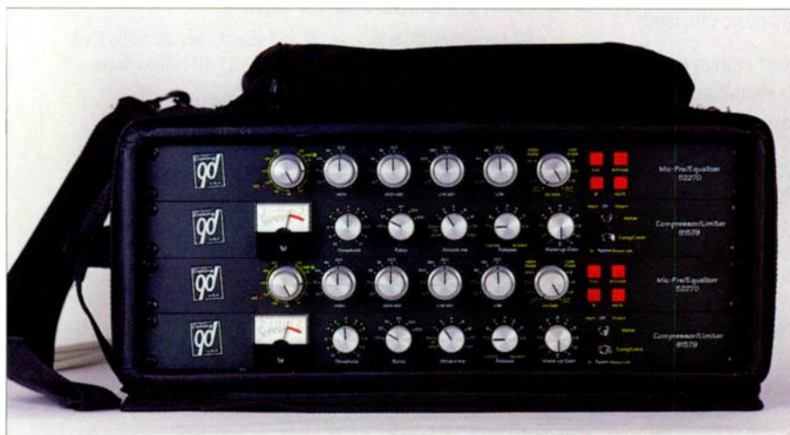
The Daking 52270 mic preamp/EQ is available in two configurations; shown here is the 1U horizontal configuration. The vertical, "lunchbox" version holds up to four modules. The six dual-concentric controls adjust the input levels, high- and lowpass filter cutoff frequencies, and EQ center frequencies.
