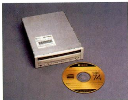
CD-R drives, such as this Ricoh 1420C, have rapidly gained in popularity as the drives and blank discs have become more affordable.
