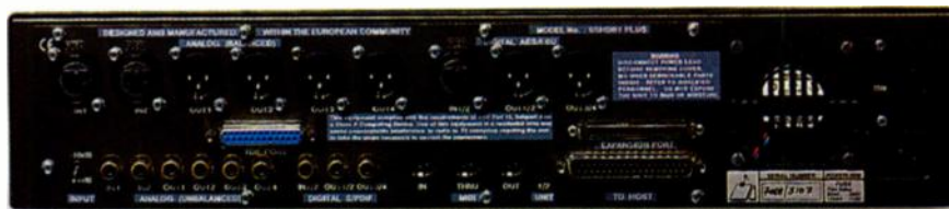
Soundscape's SSHDR1-Plus is one of the few hard-disk recording systems that includes a TASCAM TDIF port. You also get unbalanced analog I/O and S/PDIF digital I/O.
