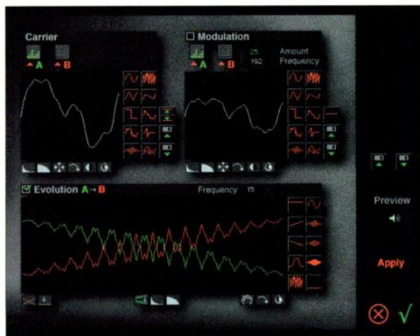
FIG. 5: The Procedural window is a 2-operator FM synthesizer with real-time interactive controls. The two operators can be carrier or modulator. The Evolution display controls the transition from A to B, with ten preset crossfade curves. Note the drag-controlled tools, such as the Hand and Rotate tools (lower right).
