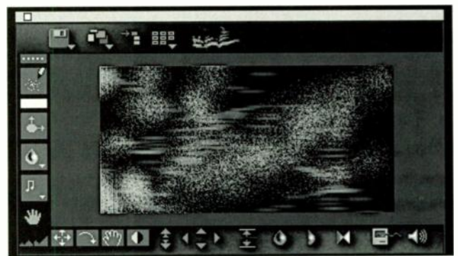
FIG. 3: In the Filter window, you can "paint" filters onto a sound with the Brush/Pencil tools. Every brush/pencil stroke produces a blue line that passes sound at a specific frequency. Unpainted black areas let through no sound. Time is on the x axis and frequency is on the y axis.
