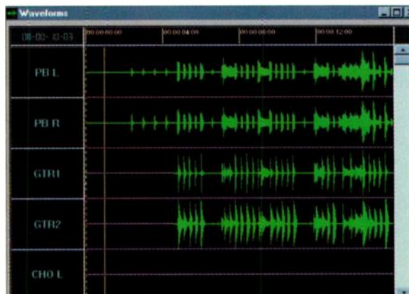
FIG 2: The Waveform window displays the digital audio data contained in all eight tracks simultaneously. Unfortunately, graphical editing with copy, cut, and paste isn't allowed.
