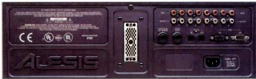
FIG. 1: The XT20's rear panel offers both -10 dBV, unbalanced I/O (through RCA jacks) and +4 dBu, balanced I/O (via a 56-pin EDAC connector). ADAT Optical connections are also provided, as well as two discrete jacks for the LRC and a punch in/out pedal.
