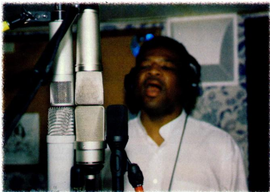
Five mics were clustered together to capture singer-songwriter Johnny Staton singing “Amazing Grace” for EM ’s cardioid condenser mic comparison.
