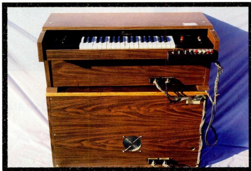
With the addition of the M1 remote, a Chamberlin M1 (seen here sitting on top of the remote) could play four simultaneous tracks and access sixteen sounds from one keyboard.
