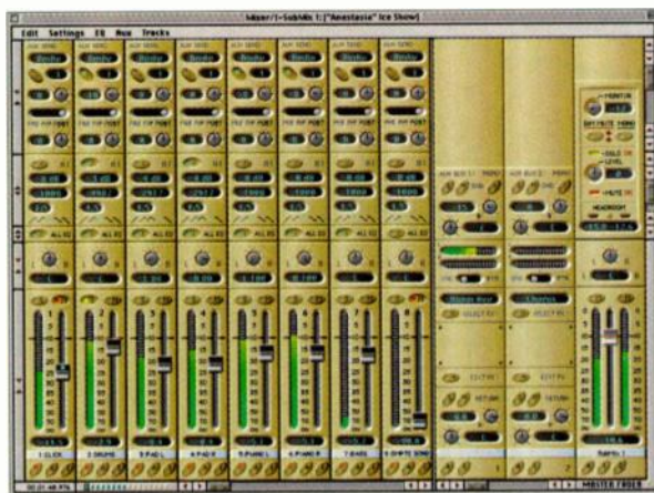
FIG. 5: The Mixer window is comprehensive, offering a long-throw fader, a level meter with headroom indicator, solo and mute buttons, a pan pot, EQ controls, an aux-send section, an insert section, and record-enable and automation buttons.
