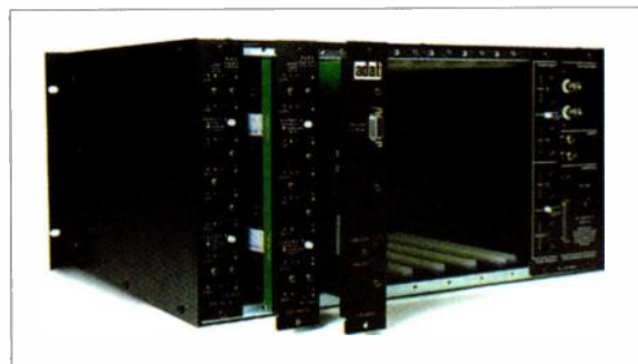
FIG. 3: The Modular Expansion Chassis (MEC) can accommodate up to five I/O modules. Three modules are currently in production: the A8iT-24 8-channel, 24-bit A/D interface, the A8oT-24 8-channel 24-bit D/A interface, and the EDS-ADI-01 8-channel ADAT optical interface. Future modules will provide AES/EBU and TASCAM TDIF I/O.
