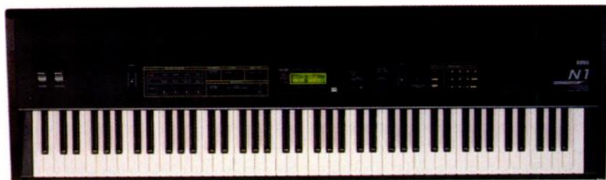
Korg's N1 delivers a wealth of good sounds; solid effects; 88 keys; weighted action; and an arpeggiator. Instead of having an onboard sequencer, it offers a computer interface for use with software sequencers.
