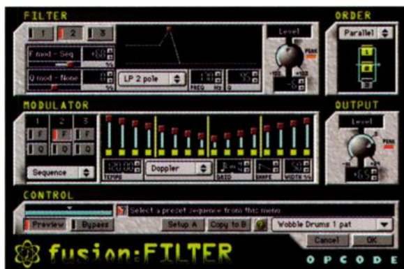
FIG. 3: The most complex plug-in of the fusion: EFFECTS series, FILTER offers a number of resonant filters and LFOs, in addition to a very cool Pulse Sequencer.
