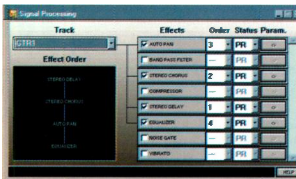
FIG. 4: Track effects are assigned using the Effects Connection dialog box. Each track can have its own chain of effects with individual parameter settings.
