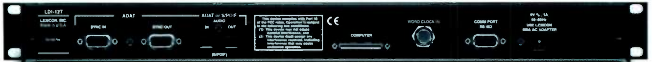
FIG. 2: The rear of the LDI-12T interface offers optical Toslink connections for 8-channel ADAT or S/PDIF formats and provides serial connections for ADAT sync and machine control.
