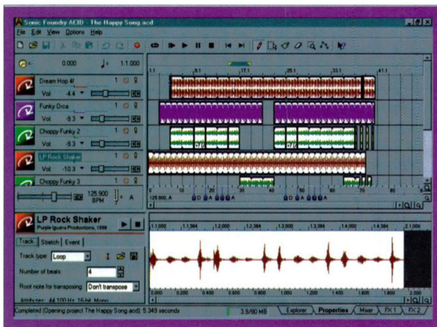
FIG. 2: To ACID-ify an audio file, an extra chunk of data is added that contains settings specific to ACID. These settings are accessed via the Properties tab at the bottom of the accessory panel.
