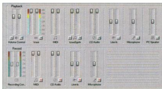
FIG. 4: Digital Orchestrator Pro 's Audio System Mixer uses a sound card's multimedia mixer for controlling input/output settings and for monitoring audio record and playback levels.
