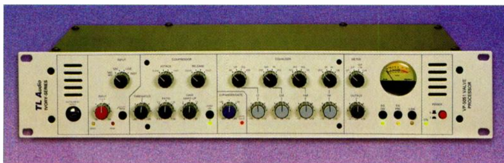
The 5051 Mono Valve Voice Processor is a hybrid tube/solid-state preamp that adds tube coloration to the signal while keeping a relatively clean signal path. Added features include a 4-band equalizer, a compressor, and an expander/gate.
