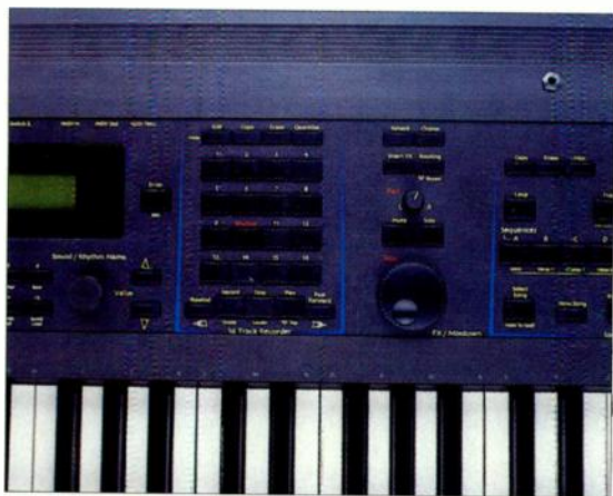
FIG. 3: The sequencer, which Ensoniq dubs "16 Track Recorder," has dedicated track buttons with LEDs that light up to indicate that the associated tracks contain data. The section to the far right shows four of the eight lettered Sequence buttons; you can assemble up to eight sequences per song. Notice the labels below the buttons, which indicate Intro, Verse 1, and so on.
