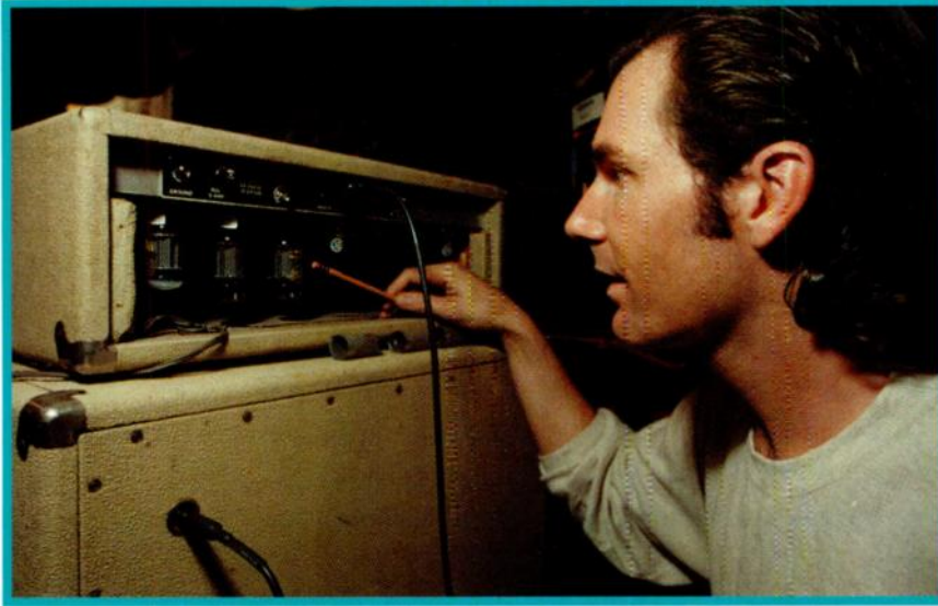
Matt Blackett taps on the preamp tubes of an old Fender amp to find the microphonic one.
