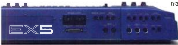
The EX5 with SCSI and analog expansion boards installed.
