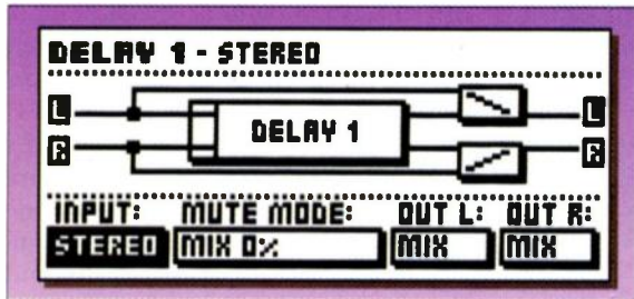
FIG. 3: Each individual algorithm's ins and outs can be separately defined, allowing complete flexibility for feeding and returning signals within the effects chain.
