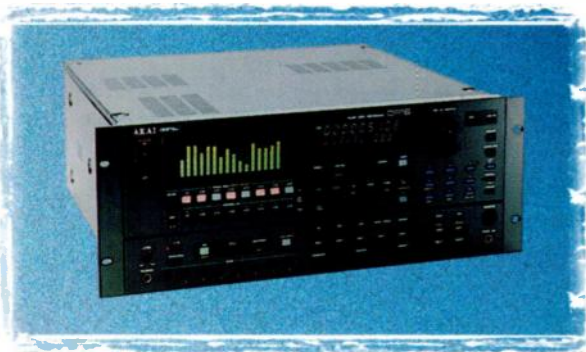
DeAngelis brought his own Akai DR-16 hard-disk recorders into the studio, and they were essential for capturing live tracks.
