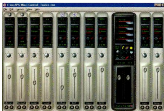
FIG. 1: E-mu's E-Control Mixer software lets you route audio and provides access to the effects. In the program's Mixer Control window, the analog input strips are marked "A," and the S/PDIF inputs are marked "D." The "Midi" strips accept signals from the onboard synths and feed the main MIDI input strip.
