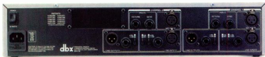
The rear panel of the dbx 586 provides mic and line/instrument inputs, as well as separate 1/4-inch insert send/return jacks on each channel. Line inputs and outputs offer a choice of XLR or 1/2-inch jacks, plus level-matching switches.
