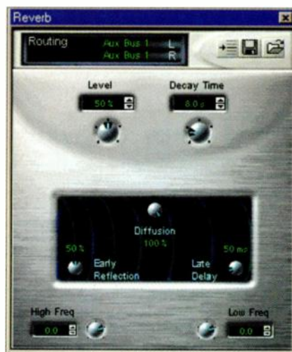
FIG. 2: The APS comes with a variety of onboard effects. This figure shows the Edit window for the reverb.
