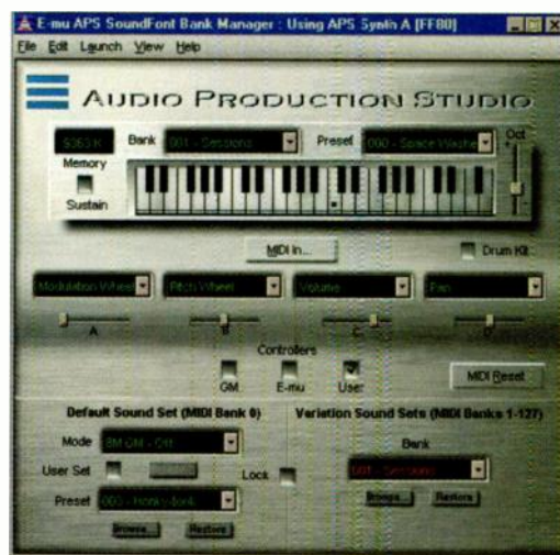
FIG. 3: SoundFont Bank Manager lets you load SoundFont files into any APS bank. You can also use this tool to audition the sounds in each bank.
