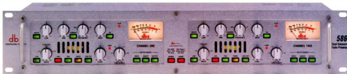
The dbx 586 dual-channel preamp is a hybrid tube/solid-state unit with several useful features. It provides a low-cut filter and 20 dB pad, 3-band EQ with sweepable mids and switchable Q (wide/narrow), and dbx's proprietary PeakPlus limiting. The switches in the center of the unit control an optional digital-output module.
