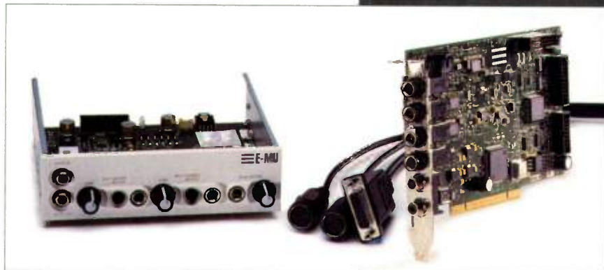
E-mu's Audio Production Studio consists of the E-Card PCI audio card, which also houses two synths; the E-Drive I/O module, which fits into a front-loading drive bay; and bundled software. A MIDI bracket provides MIDI In and Out ports on a 15-pin connector.
